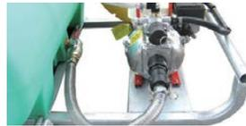
3. Detach the suction hose from pump and attach to top outlet - refer to visual
