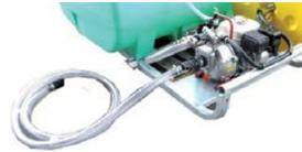
5. Place foot strainer and hose into water source - ensure the strainer is in clean water free of sludge or debris.
