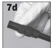
Adjust spray pattern by turning nozzle cap. Do not turn cap more than 2 turns or cap may come off allowing spray material to spray back on you.
