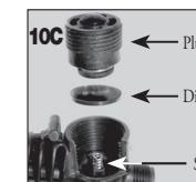
Remove plunger, diaphragm and spring. Wash diaphragm with mild detergent. Reassemble: Hold shut-off upright as shown, place spring in hole, place diaphragm on top of spring. Reassemble plunger and tighten.
