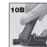
Insert notches from underside of handle into plunger grooves and turn counter-clockwise.
