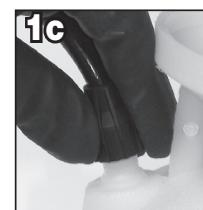
**Do:** Slide nut down over threads. Turn nut clockwise as tight as possible.
