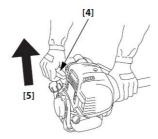
5. If the choke lever was moved to the CLOSED [A] position to start the engine, gradually move it to the OPEN [B] position as the engine warms up.
