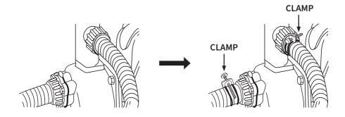
**NOTE.** When installing the joint to the pump, be sure the gasket is in place. Ensure that the hoses are securely installed or air lead will occur and water will not be drawn up.
