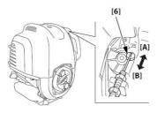
**Hot Restart:** If the engine is operated at higher ambient temperatures, then turned off and allowed to sit for a short time, it may not restart on the first pull.
