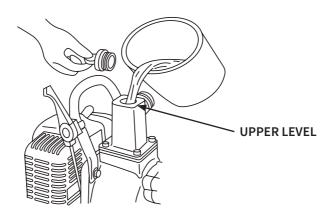
**WARNING!** Be sure that the pump is filled up with water before starting the engine, else mechanical seal damage will occur.
